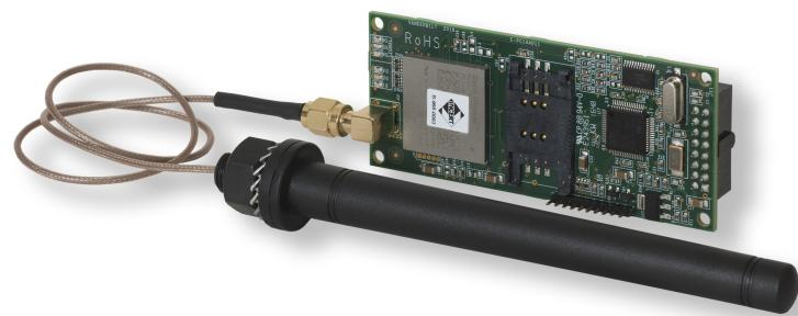
The SPCN320 GSM module can be assigned to any mobile network by the insertion of a standard SIM card. The modem is compatible with the complete range of acre intrusion panels and plugs directly on the main PCB removing the need for any additional wiring. The unit comes with an external antenna that fits on the cabinet.
